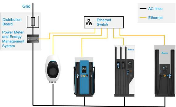
The default ModBus TCP Port is 502 on ACMAX and 5020 on UFC/SLIM.
