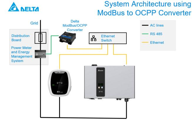
In this setup, the ModBus to OCPP Protocol Converter acts as OCPP Proxy to the OCPP Back End (if applicable)
